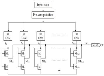
Fig. 6 Block Diagram of PB-SCPF CAM
