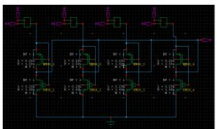
Fig. 11 Design of SCPF CAM
