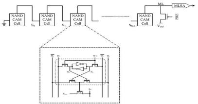
Fig. 2 Word Structure of NAND-Type CAM
