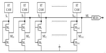
Fig. 5 Word Structure of SCPF-CAM
