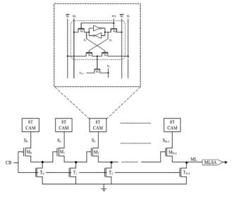
Fig. 4 Word Structure of PF CAM
