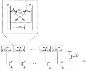
Fig. 3 Word Structure of NOR-Type CAM
